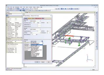
Stress, flexibility, stability, and fatigue strength analysis are performed for buried, above ground, vacuum, high pressure, high temperature, and cryogenic piping.
